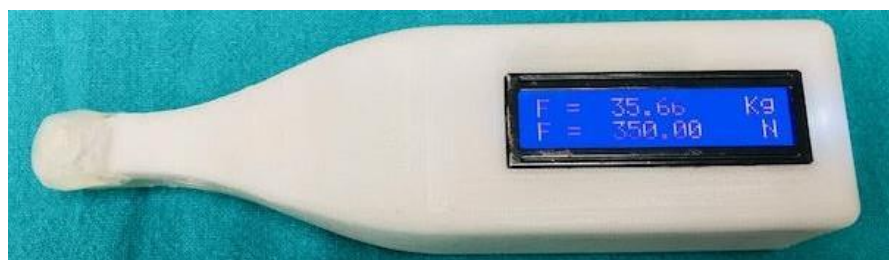
Image B: Flexiforce sensor device to record bite force
