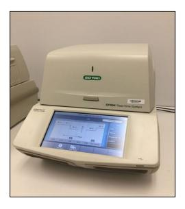
Image 6: Bio-Rad CFX 96 Thermal cycler (real-time PCR System)
